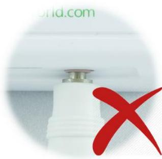
**NOTE!** Check that the sensor is inserted into the 3.5mm red jack socket to the very end. The connection is tight and you have to ensure that there is no gap between the connector of the sensor and the jack socket!
